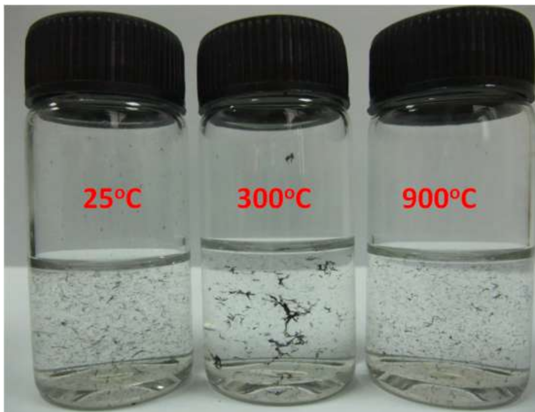
Fig. S5. Optical images of CNTs dispersed in ethanol after ultrasonic treatment for an hour. CNTs were obtained from the fibers before and after heating treatment at 300 and 900 °C in argon.
