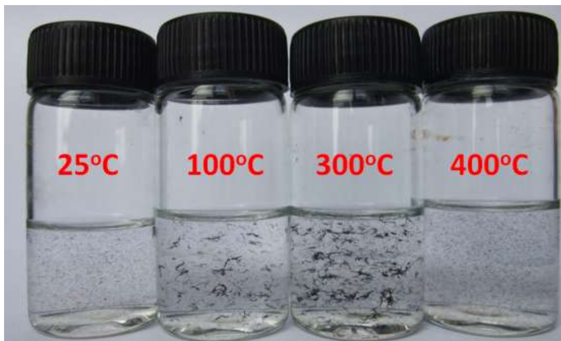
Fig. S11. Optical images of CNTs dispersed in ethanol after ultrasonic treatment for an hour. CNTs were obtained from the fibers before and after heating treatments at 100, 300, and 400 °C in air.
